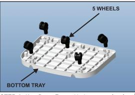
**STEP-1:** Keep Bottom Tray upside down on a soft surface to avoid scratches. Fix the Wheels on the Bottom Tray by positioning the Wheel Caps along with the holes on the Bottom Tray and pushing inside.
