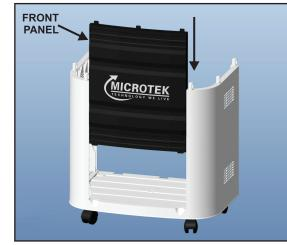
**STEP-3:** Fix the Front Side Panel by sliding between side panels in the center and pushing into the bottom panel.
