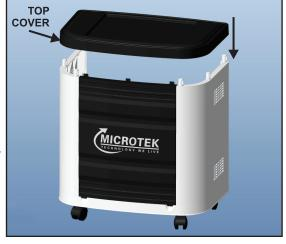
**STEP-4**: Fix the Top Cover on the Top by positioning the holes along the pipes and pushing inside.
