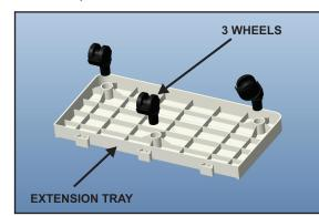
**STEP-2:** Keep Extension Tray upside down on a soft surface to avoid scratches. Fix the Wheels on the Bottom Tray by positioning the Wheel Caps along with the holes on the Extension Tray and pushing inside.
