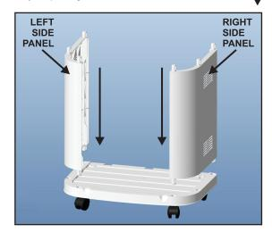
**STEP-2:** Fix the Right Side Panel and Left Side Panel on the Bottom Tray by positioning the pipes along with the holes on the Bottom Tray and pushing the pipes inside one by one.
