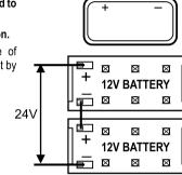
NOTE: Recommended Battery(Lead Acid Type): 24V System: 2x12V: 100AH to 200AH.
