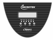
Press ON-OFF for 4±1sec to ON and OFF the PCU. Press UP-Down to scroll PCU values, press ENTER to set value.
