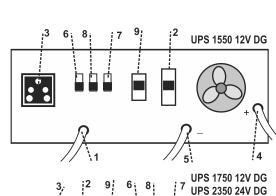
1. Mains AC Input Lead for AC input.
